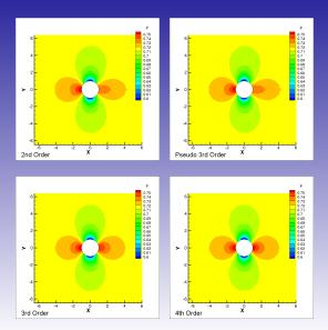
Subsonic Circular Cylinder, Grid 2 Pressure Contours
