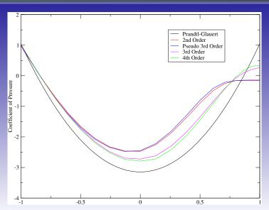
Subsonic Circular Cylinder, C<sub>P</sub> Distribution for Grid 1
