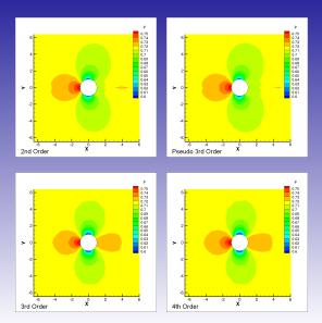
Subsonic Circular Cylinder, Grid 1 Pressure Contours
