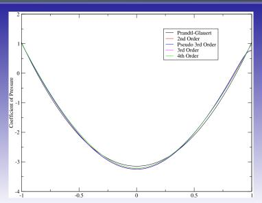
Subsonic Circular Cylinder, CP Distribution for Grid 2 Detail
