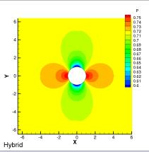
Subsonic Circular Cylinder, Grid 2 Pressure Contours with Hybrid Scheme
