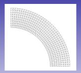
Test Same Methods Curved Boundary  $\Rightarrow$  Triangles with One Curved Side Evaluate Area Integrals with Isoparametric Mapping (Quadratic)
