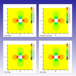
Subsonic Circular Cylinder, Grid 2 Pressure Contours (Detail)
