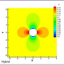
Subsonic Circular Cylinder, CP Distribution for Grid 2 with Hybrid Scheme
