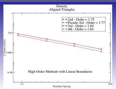
Supersonic Annulus, Error in Density from Aligned Triangles (Coarsest Grid)
