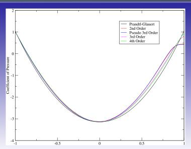
Subsonic Circular Cylinder, C<sub>P</sub> Distribution for Grid 2
