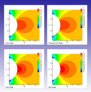
Subsonic Circular Cylinder, C<sub>P</sub> Distribution
