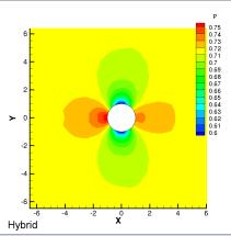
Subsonic Circular Cylinder, Grid 1 Pressure Contours with Hybrid Scheme
