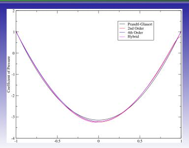
Subsonic Circular Cylinder, CP Distribution for Grid 2 Detail with Hybrid Scheme
